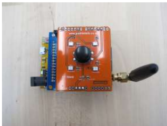
Figure 6 – View from above of PTT board
