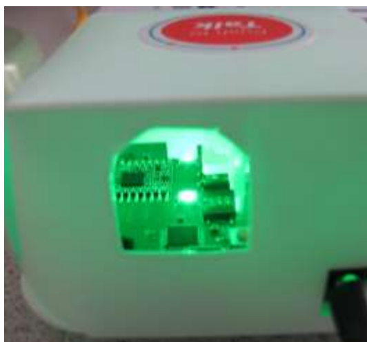
Figure 11 – PTT button in case with green indicator
